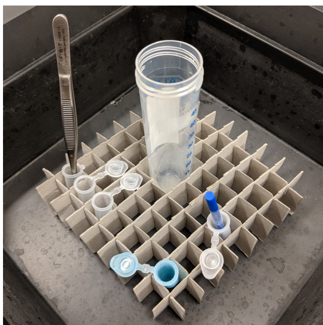
Figure 3. Photograph of set-up for grinding frozen pellets. Fill an ice bucket and conical tube with liquid nitrogen. Cool pestle in a microcentrifuge tube and use it to grind the frozen sample. To cool the sample, use forceps to grip a microcentrifuge tube, and use it to transfer liquid nitrogen from the conical tube to the sample.
